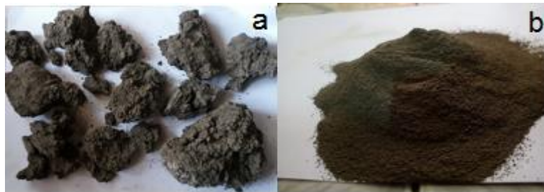
Fig. 2 Textile sludge: (a) before crushing; (b) after crushing (Abbas et al., 2021)
