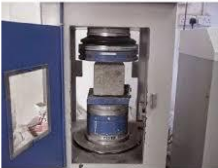
Fig.7. compressive strength test.
